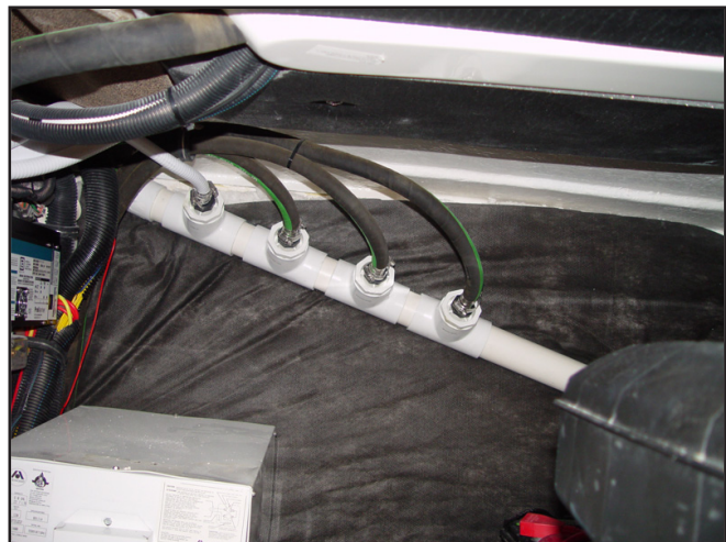
Drain Manifold in Engine Compartment
