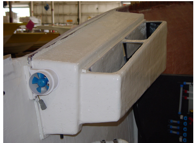
Engine Compartment Blower and Vent Baffle
