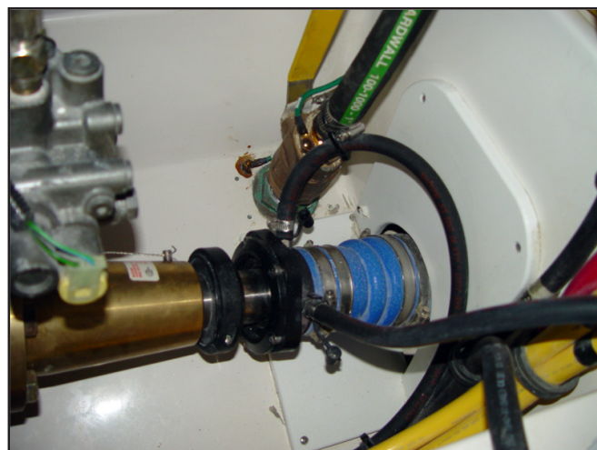
Dripless Shaft Seal, Bonding Connection and Water Hose
