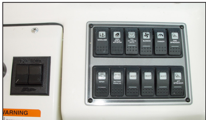
Port Helm Switch Panel
