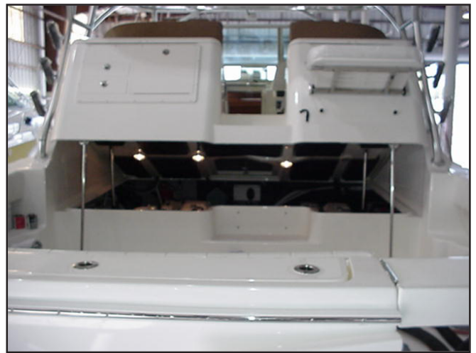
Raised Bridge Deck, Hatch Lifters and Safety Struts
