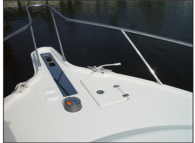
Deck Hardware, Bow Rail and Windlass
