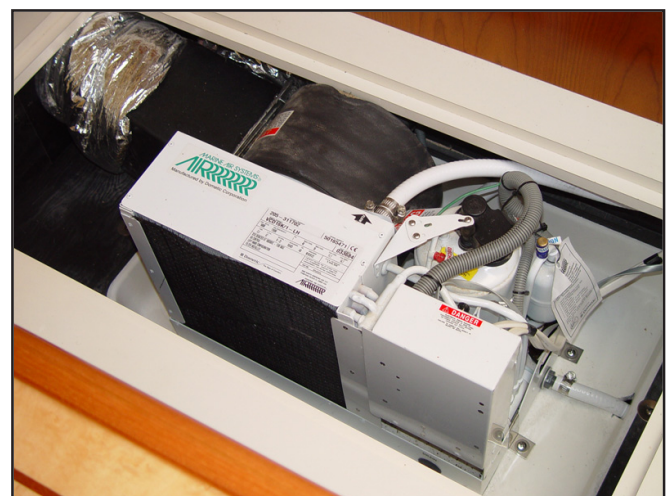
Cabin Air Conditioner and Drip Pan Drain Hose
