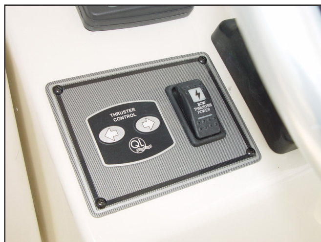
Bow Thruster Control Panel
