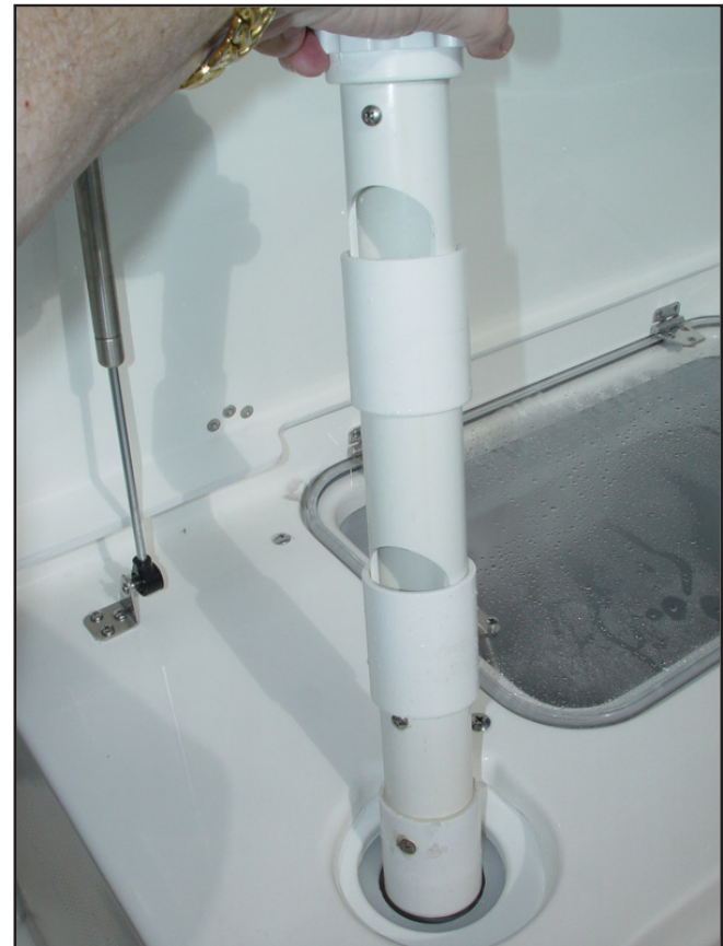
Baitwell Overflow Tube and Adjustable Valves
