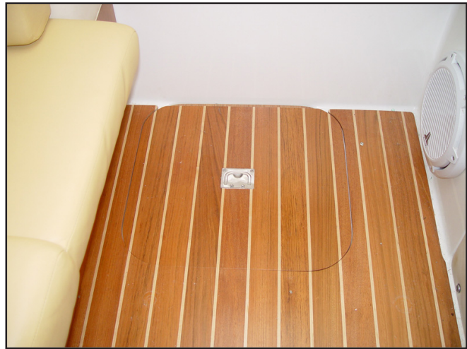
Cherry and Maple Cabin Sole and Access Hatch to Cabin Sump Pump and Forward Bilge Pump
