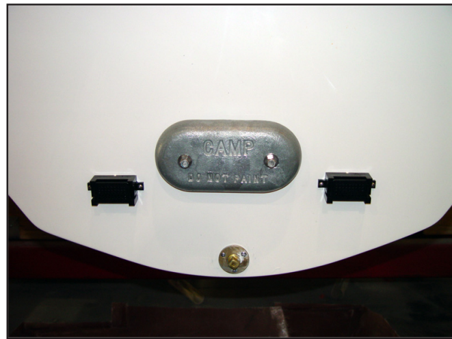
Transom Zinc Anode and Active Corrosion Anode and Cathode
